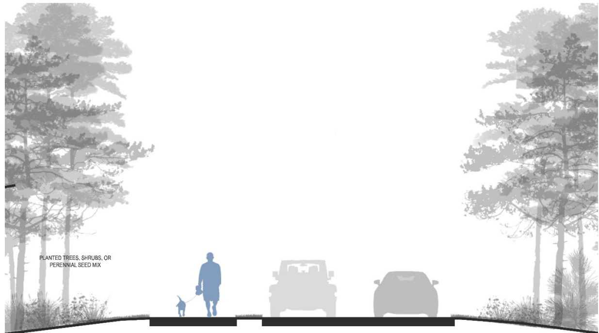
Proposed 10' Multi-Use Path next to Existing Roadway (Consistent with the Initial Report)
